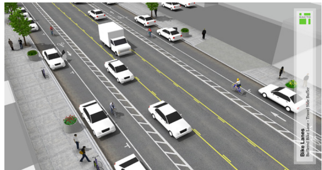
Figure 5 – Buffered Bike Lane Illustration: Travel Side Buffer
