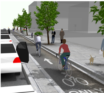
Figure 9 – One-Way Protected Cycle Track Illustration: Raised Curb and Parking Buffer
