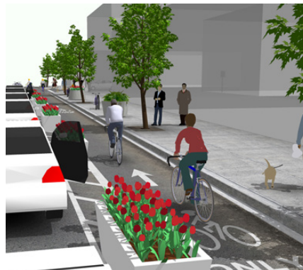
Figure 10 – One-Way Protected Cycle Track Illustration: Planter and Parking Buffer
