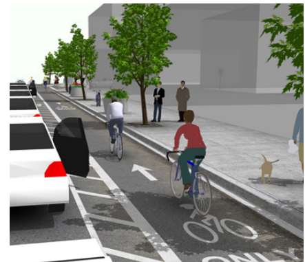
Figure 11 – One-Way Protected Cycle Track Illustration: Parking Buffer
