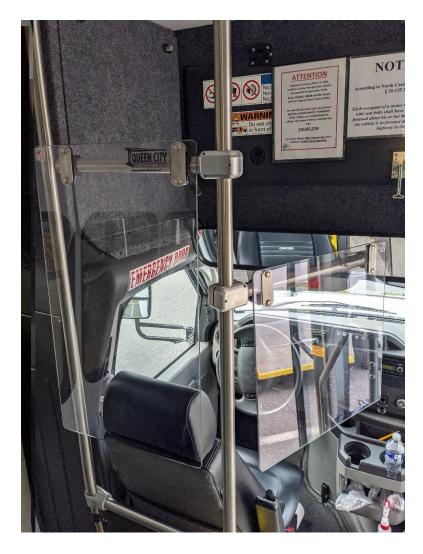
Our shielding systems far surpass others in the market in terms of quality and performance. Made only from American made materials including 1/4" thick polycarbonate, food grade stainless steel, and aircraft grade aluminum, our systems are built to last.
