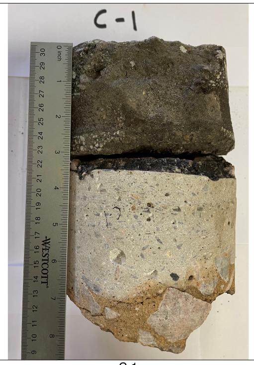
C-1 Asphalt Thickness (3½") Concrete Thickness (4") Stone Base (12")
